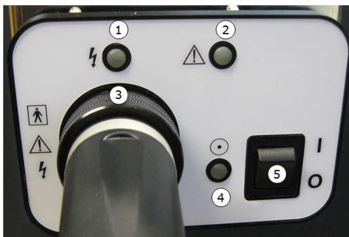
Fig. 5. TMS II Stimulator front panel
