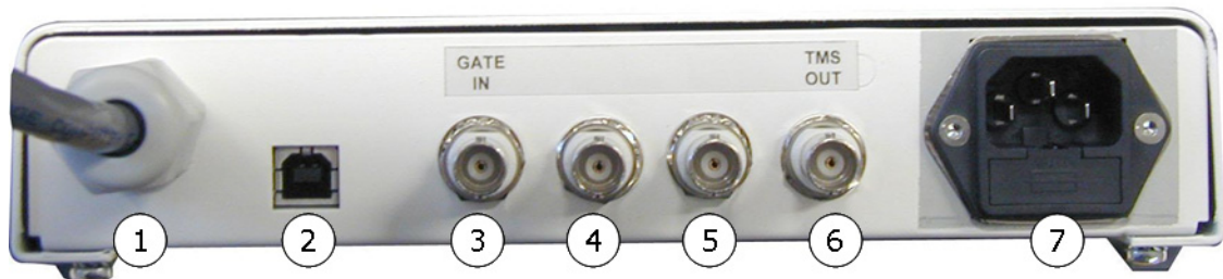
Fig. 158. Nexstim EMG power unit connections
